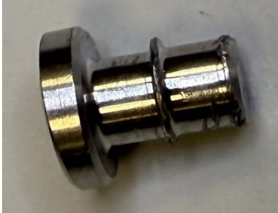
Figure 5: Example picture of Femoral Augment screw without thread
